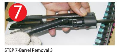
3. Pull the barrel and remove from the slide
