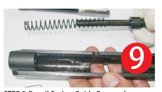
STEP 9-Recoil Spring Guide Removal Pull off the recoil spring guide with the spring from the slide
