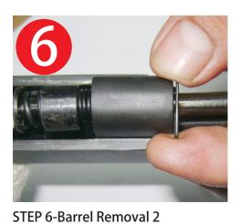
2. Insert a pin at the recoil spring guide's hole to stop a backward motion. You can use any pin as long as it fits the hole.
